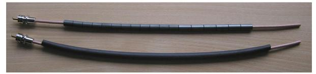
6. Cut a piece of 35cm heat shrink tubing 9/3mm. Place the ferrites in the center of the cable, leaving approx. 8cm on both sides. Pull the heat shrink tubing over the ferrites. This results in an overlap of approx. 3cm on both sides.
